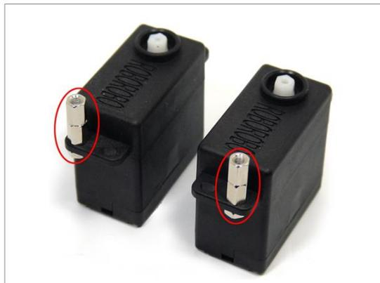
3. Connect two 7mm support and fix them the DC motor using nuts.
