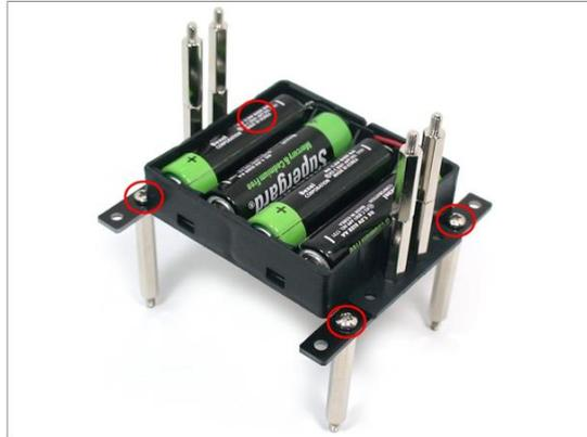
2. Tighten 35mm supports that are located on the battery case.
