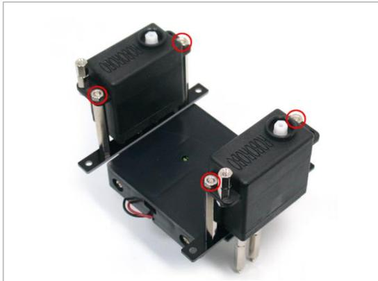
4. Fix the 8 hole frame connecting 35mm support to the DC motor using nuts.
