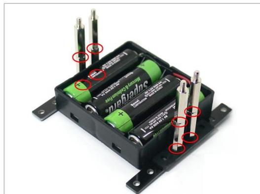
1. Locate 8hole frames on the battery case and tighten 20mm supports using bolts.
