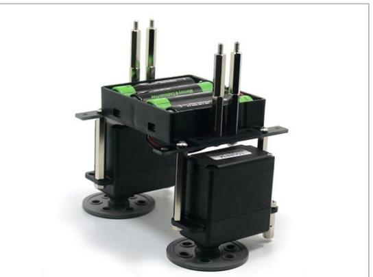
5. Insert wheel guides to the DC motor's pivots.
