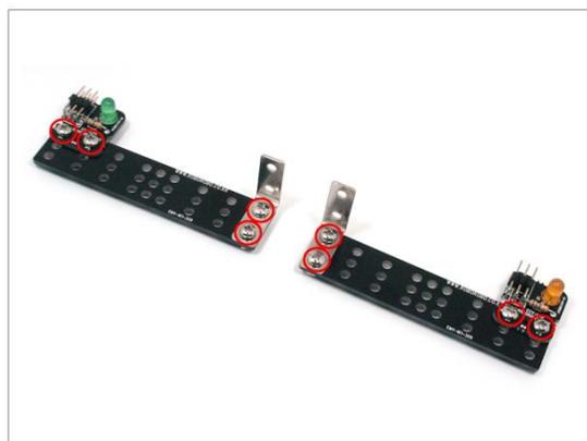
7. Locate the LED board and the L2X2 frame on the middle frame and tighten them using bolts and nuts.
